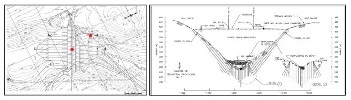
Figure 1.a) Plan view of the Denis-Perron dam, 1b) Longitudinal section of the valley in the central dam axis
